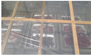
Fig. 1. Drying of red amaranth in greenhouse-based solar dryer
