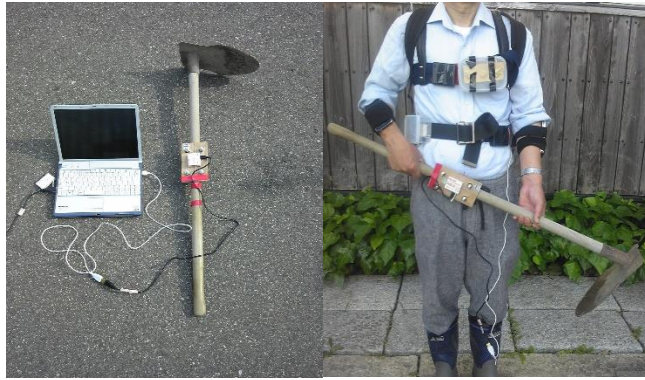
Fig. 2. A subject equipped with measuring modules and knapsack with laptop PC connecting to various modules.
