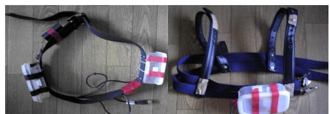
Fig. 1. Microcomputers with various devices, store-bought sensing modules, and original vest-shaped and belt-shaped WSs.
